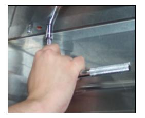
Removing the hole cover weldment
